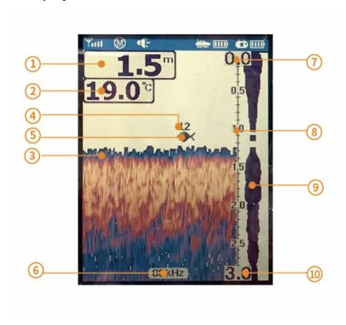
1.Water Depth 2. Water Temperature 3. Bottom Contour 4. Fish Depth 5. Fish Icon .6. Sonar Frequency 7 Lower Limit 8-Depth Scale 9.Upper Limit 10.DTS single
